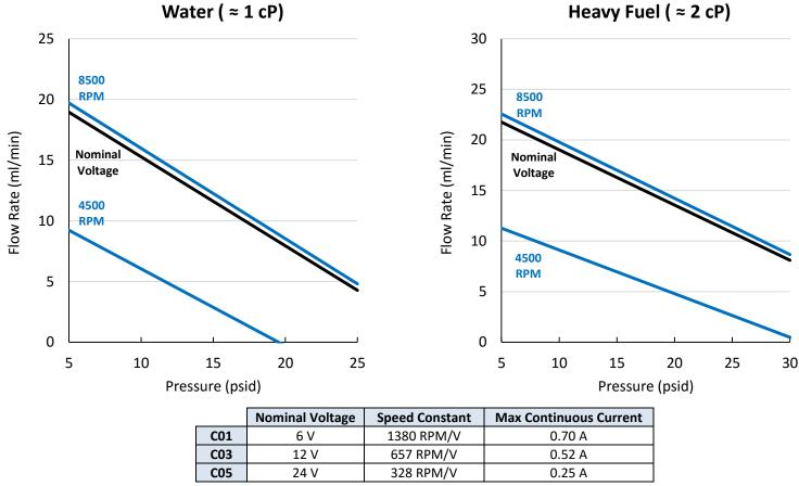
NOTES: Dashed lines indicate <u>intermittent</u> operation; speed constant may vary at higher pressures; RPM flow lines indicate performance at typical maximum and minimum speeds;
